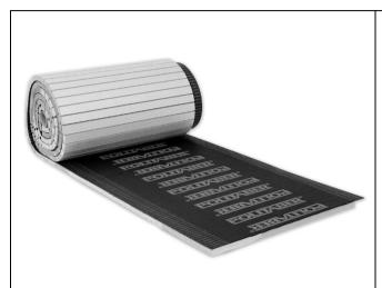
**ChovATERM**® is a complex formed by a thermal insulation, with strips cut from XPS panels—**ChovAFOAM**, thermally adhered to bituminous sheets of modified with elastomers bitumen - **POLITABER**.
